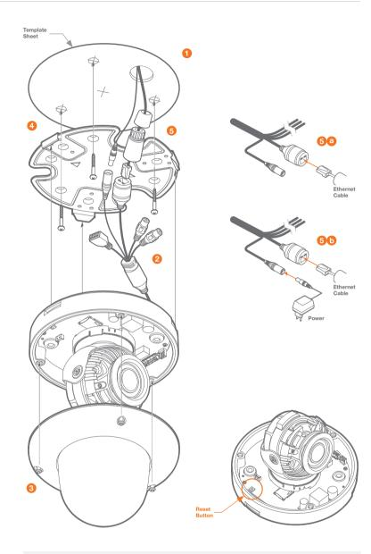
Resetting the camera: To reset the camera, use the tip of a paper clip or a pencil and press the reset button. Pressing the button for five (5) seconds will initiate a camera-wide reset of all the settings, including network settings.
