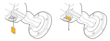
NOTE: Maximum SD Card size supopoorted: 64GB. When inserting the SD card into the card slot, the SD card's contacts should be facing upward, as shown in the diagram.
