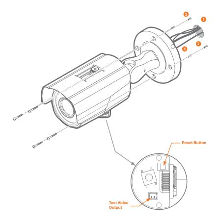
Resetting the camera: To reset the camera, use the tip of a paper clip or a pencil and press the reset button. Pressing the button for five (5) seconds will initiate a camera-wide reset of all the settings, including network settings.
