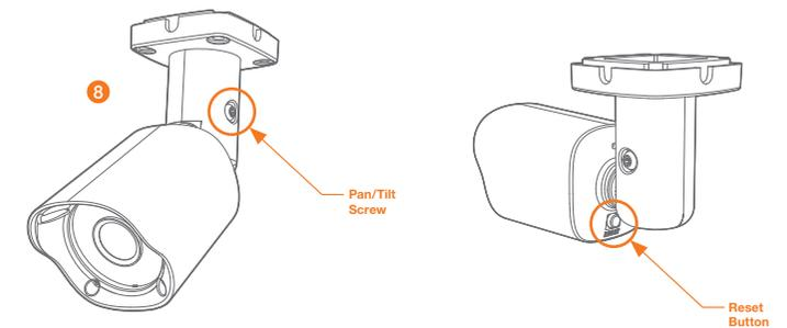
**Resetting the camera:** To reset the camera, use the tip of a paper clip or a pencil and press the reset button. Pressing the button for five (5) seconds will initiate a camera-wide reset of all the settings, including network settings.
