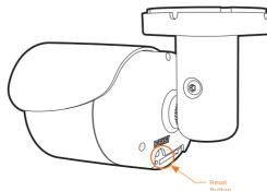
Resetting the camera: To reset the camera, use the tip of a paper clip or a pencil and press the reset button. Pressing the button for five (5) seconds will initiate a camera-wide reset of all the settings, including network settings.
