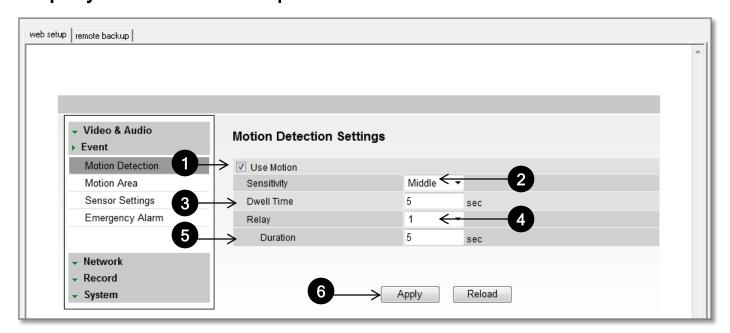
The Motion detection feature allows the MEGAPIX camera to detect motion and trigger an alarm. To set the camera to send e-mail notifications for every motion triggered alarms, see page 50.
