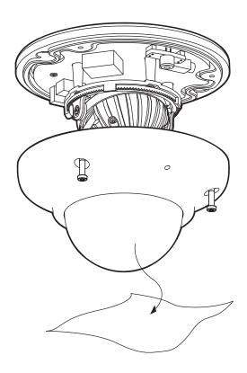
To achieve desired view direction and orientation, rotate 3-axis gimbal. To fix the setting, tighten the tilt stopper screw.
