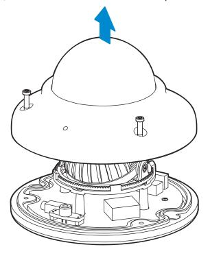
To re-attach the dome to the camera base, match the one screw hole on the dome cover and camera bottom specially.
