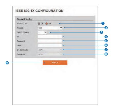
The feature is needed when connecting the camera to the network protected by the IEEE 802.1X.
