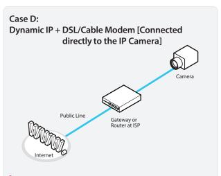
To connect the IP Camera directly to a modem, power down and reset the modem. Leave the modem powered down until configurations are finalized with the IP Camera and the IP Camera has been connected correctly to the modem. Then power on the modem, followed by the IP Camera.
