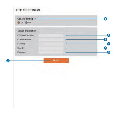
To transfer / save the image to the relevant sites through FTP, then FTP needs to be setup.
