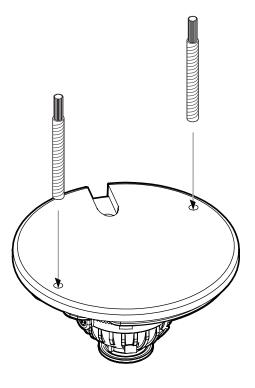
3 Insert the 2 mount bolts into bottom case of camera.
