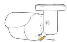
**NOTE:** When inserting the SD card into the card slot, the SD card's contacts should be facing upward, as shown in the diagram.
