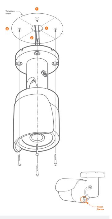
Resetting the camera: To reset the camera, use the tip of a paper clip or a pencil and press the reset button. Pressing the button for five (5) seconds will initiate a camera-wide reset of all the settings, including network settings.
