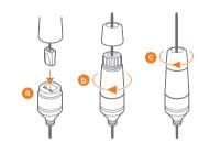
Note: To ensure moisture seal, make sure the o-ring is in place between (a) and (b). In extreme environments use of an outdoor rated sealer
