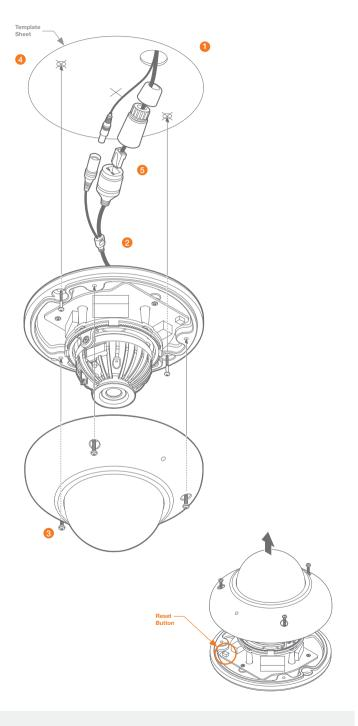
Resetting the camera: To reset the camera, use the tip of a paper clip or a pencil and press the reset button. Pressing the button for five (5) seconds will initiate a camera-wide reset of all the settings, including network settings.
