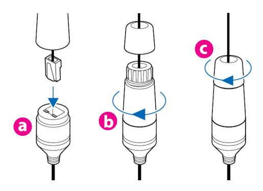
NOTE: To ensure moisture seal, make sure the O-ring is in place between (a) and (b). In extreme environments use of an outdoor rated sealer is recommended.
