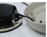
As shown in the diagram, the MEGAPIX camera comes with a safety wire attached. The safety wire will secure the dome to the camera module during the installation process.
