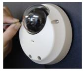
8 Tighten the four locking screws.
