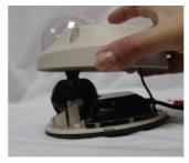
Using the supplied T10-M3x15.0 Allen Key, loosen the four security screws. Carefully remove the dome cover.
