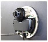
9 Pull wires through and make connections. Refer to "Network Connection" for further explanation. 6 Mount the camera to the wall or ceiling using the screws provided with the camera.
